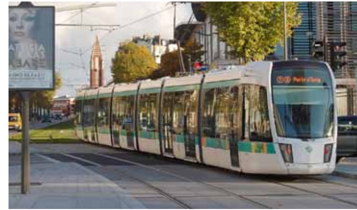
The T3 tram line is one of four tram lines in Paris that exemplify the Rapid Streetcar mode. Typical of European street trams, it uses articulated, higher-capacity trains and exclusive right-of-way. Although Paris historically had an extensive network of street trams, predating its Metro system, its modern tram lines have all been constructed since the 1990s.
