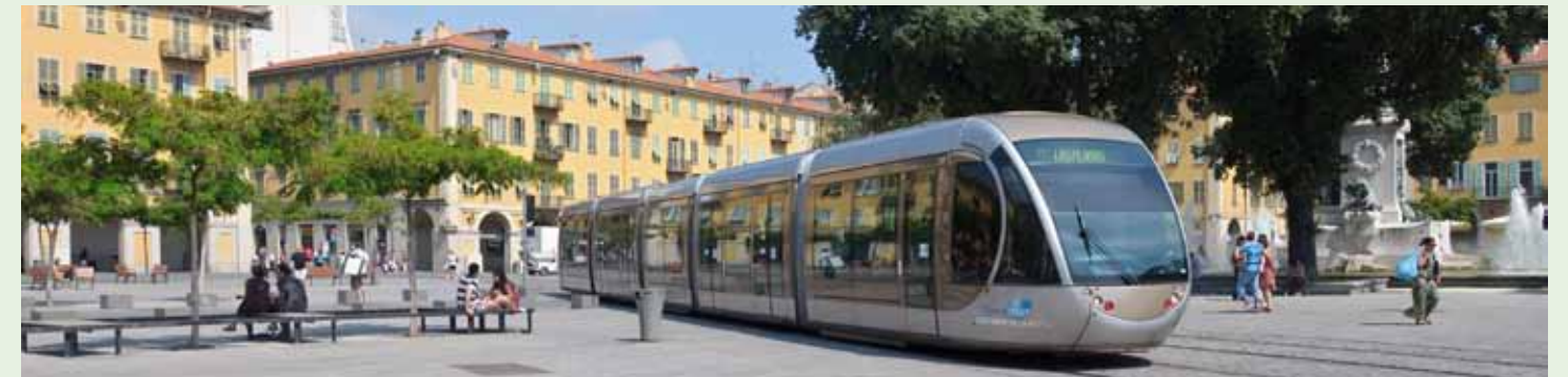
T1 tram in Nice's Place Giribaldi, where the tram runs without overhead wires, using batteries for a short section.
