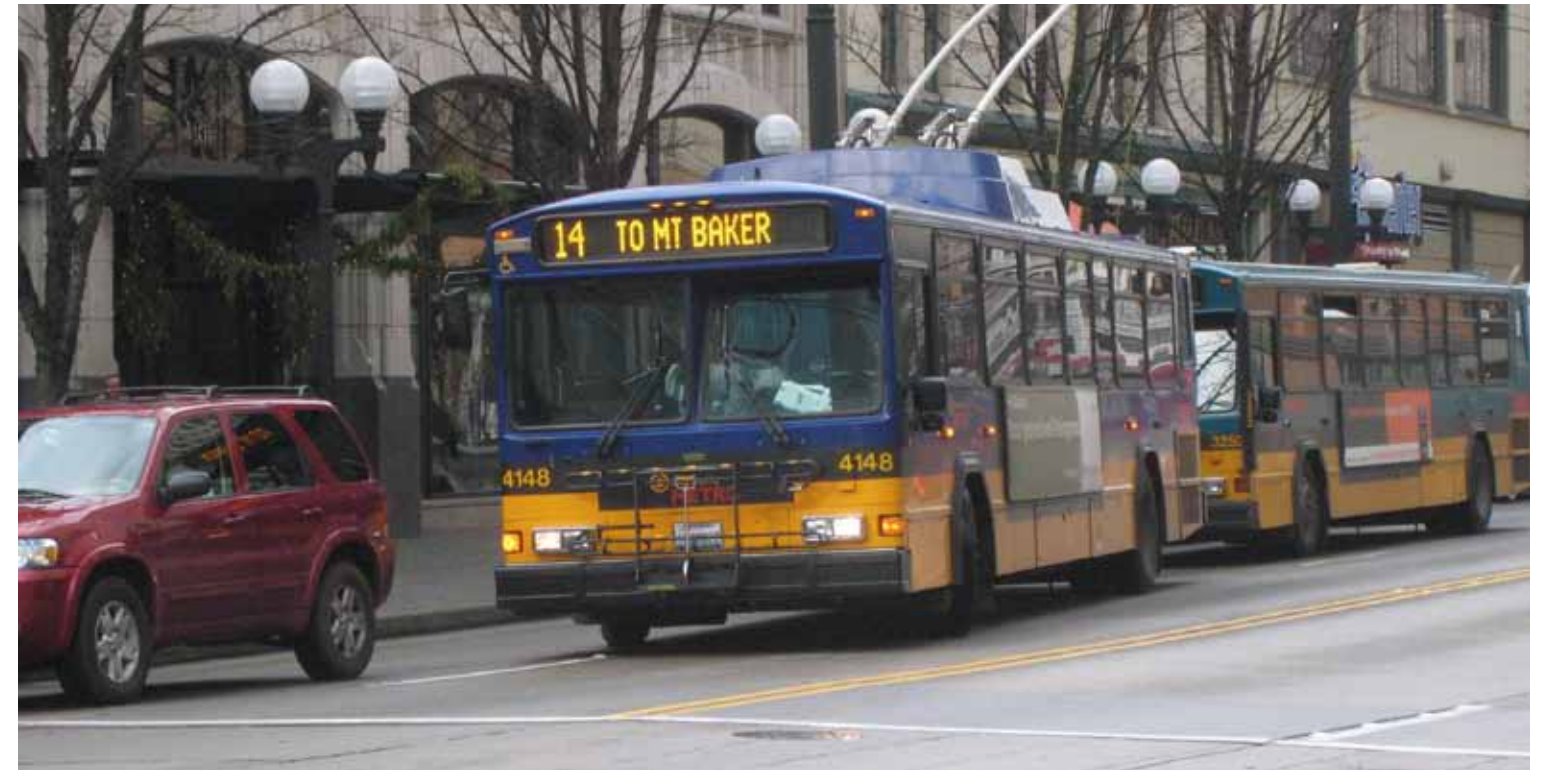
King County Metro operates 14 electric trolley bus routes using 70 miles of two-way trolley wire and 159 vehicles.
