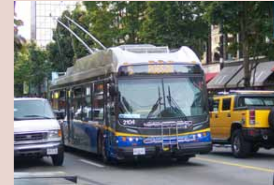
A Translink electric trolley bus in Vancouver, B.C. This is a 40' New Flyer vehicle with battery auxiliary power allowing off-wire operations.
