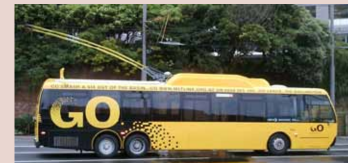
Wellington NZ carbon fiber poles reduce "jumping" wires or dewirements. This vehicle is produced by Designline Vehicles.
